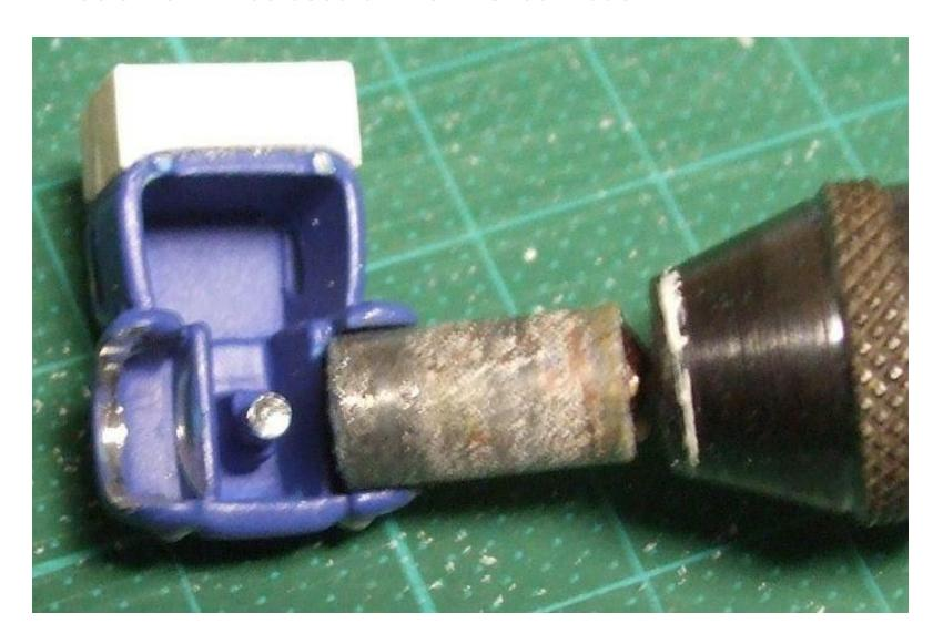
7. The rear window of the sleeper is filled with styrene, and new side windows for the sleeper are drilled and formed with a small file.
